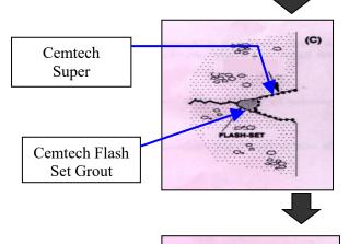
3. Stem the flow of water by plugging the back of the cutting as illustrated with Greenseal Flash Set Grout.
