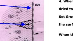
4. When the coating of Cemtech Flash Set Grout has dried to a tacky consistency, fill the cavity with Flash Set Grout again ensuring the same is compacted back to the surface.
