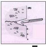
2. Chisel out defective area to a depth of approximately 50mm.
